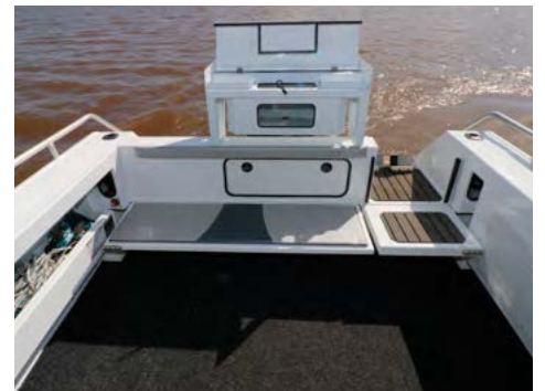
Rear 3/4 flush folding rear lounge w/ backrest, transom hatches, battery access are standard.
