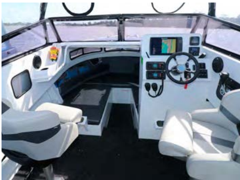
Two Bolster Seats & Air Ride pedestals (seat box for PRO DECK™) & Passenger side console.
