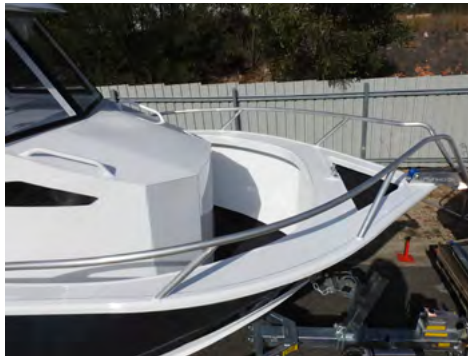
Walk around Cabin with raised casting deck, aluminium anchor well, handrails and bowroller.
