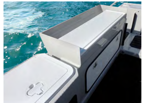
OPTIONS: Live Well with viewing window and hatch. Low Profile Bait Board.
