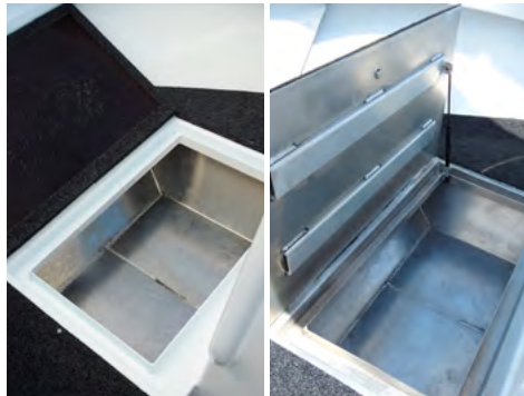
Forward deck with large storage bay with drainage.
